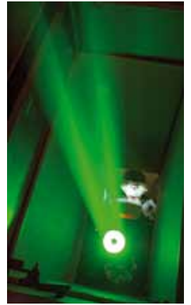
Agnes Scott Koleji ve Georgia Institute of Technology işbirliği ile ABD'de kurulmuş olan eğitim amaçlı LİDAR sistemi http://eosl.gtri.gatech.edu/Capabilities/RemoteSensing/LidarResearch/LidarProjects/tabid/220/Default.aspx
